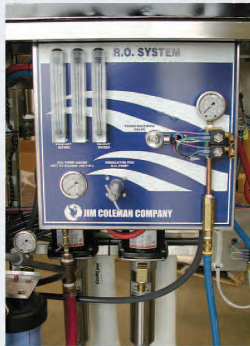
Spot-Free Rinse as installed "on-board" the Power Pack and Super Saver Car Wash Systems.
