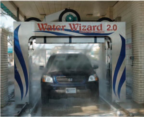
The scrubbing action oscillating nozzles sweep back and forth over the entire vehicle as the wash gantry passes over the vehicle.
