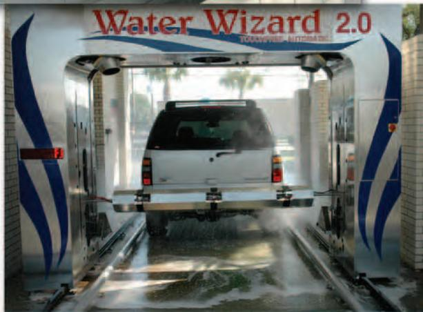
The specially designed wash boom with high impact, zero degree oscillating nozzles will rotate and attack the dirt on the front and rear of the vehicle. An additional "Bug Pass" can be programmed, front and rear, to provide extra cleaning when seasonal changes require it.
