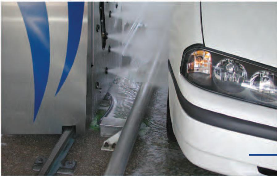
*Zero degree oscillating nozzles deliver an extra blast of cleaning power.*
