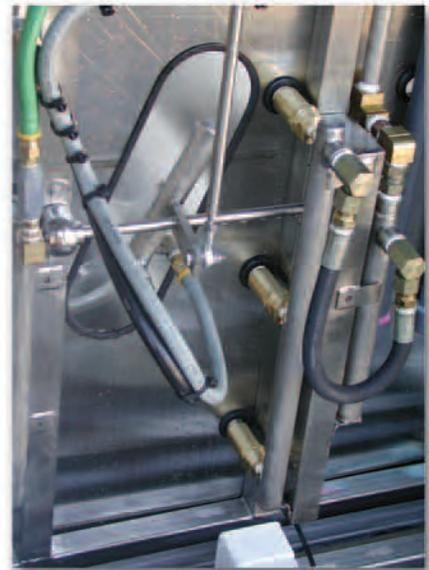
*Zero degree Rocker Panel nozzles oscillate internally creating a 20-25 degree spray pattern with no moving parts.*
